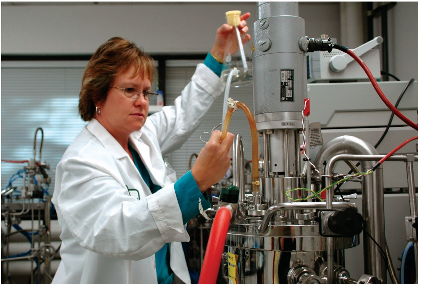
A Bayer CropScience scientist employs a fermentation device at the company's R&D biological products lab in Davis, Calif. Fermentation is the process by which biological products are produced for agriculture, much like making beer.
