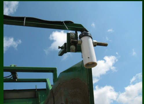
Automatic height control for the unloading conveyor
